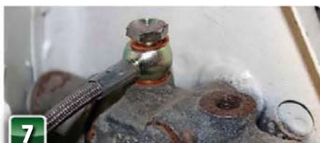
7 The new pipes use a banjo bolt arrangement, with the relevant bolts and copper washers arranged as shown. Bolting the new pipes into the PWDA valve is tricky with the servo in place, as the new banjo bolt fixings are bulkier than the originals. You may need to undo the servo fixings on the bulkhead to move it out of the way.
