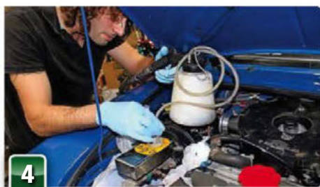
4 To minimise fluid loss, we removed all the fluid from the master cylinder reservoir using a vacuum-type bleeding tool, although you could use a syringe. Some fluid loss is inevitable, so put something underneath the servo unit to absorb it, as shown here.
