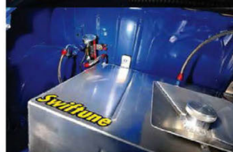
Aluminium fuel cell fitted inside the boot.
