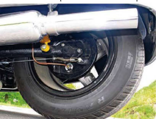
Single-sided rear suspension arrangement using one trailing arm attached to modified subframe.
