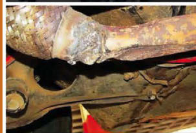
A very squashed exhaust downpipe.
