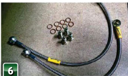
6 Here are the new pipes, complete with banjo bolts and copper washers. Fit them in the same orientation as the old rigid ones. The longer braided hose is fitted to the position closest to the engine on the PWDA valve, and furthest forward on the master cylinder.
