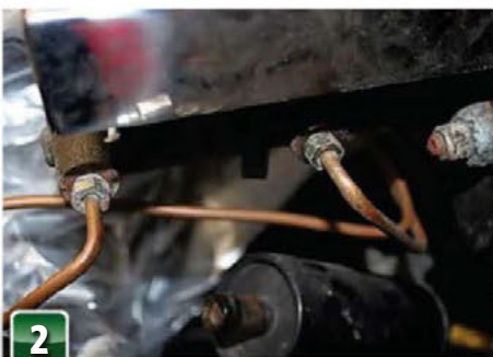
2 The two pipes run from the brake master cylinder to the PWDA valve on the bulkhead. Here are the two positions on the master cylinder.
