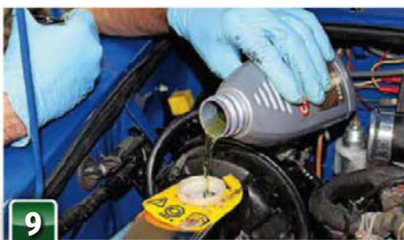
9 Now it's a case of refilling and bleeding the whole system until there is no air remaining. Once this is completed, replace the master cylinder cap, remove anything you've used to absorb stray fluid and check for leaks. That's job done!
