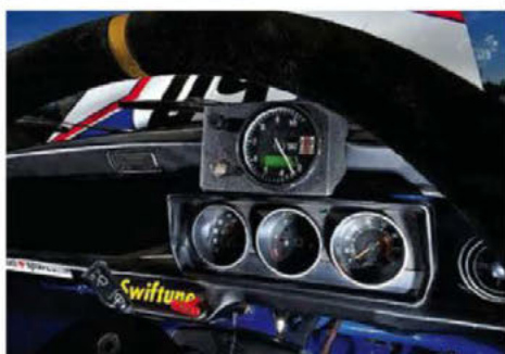
Trick new Stack gauge is housed in a replica version of the original Longman rev counter pod.
