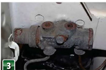
3 And here's where the pipes fit onto the PWDA unit mounted to the bulkhead. This is the valve fitted to a partially-stripped car for clarity. The servo unit makes these fixings quite tricky to reach.
